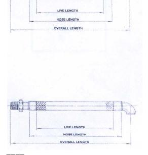
Note: This is the live length of the assembly (I.e. between the braid collars), not the overall length.
